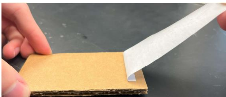
Figure 4. Image of a Passing Label Remaining Adhered Throughout The Full Peel
