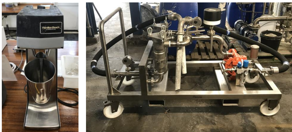
Figure 6. Left: Hamilton-Beach blender. Right: Loop-filtration test set-up.
