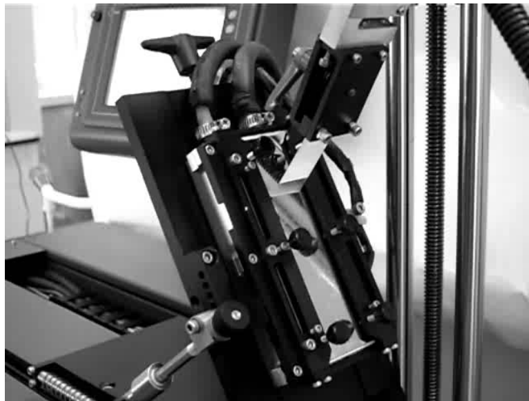
Figure 3. An experiment where the peeling angle is 60^\circ , using Equation (2), A = B = C = 60^\circ .
