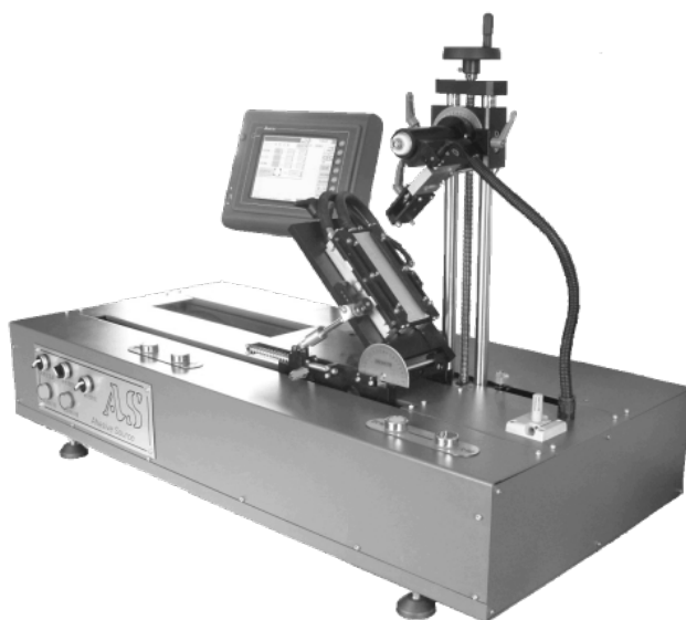
Figure 1. The multifunctional peel tester used for this study that is capable of evaluating the peel force under varying angle, rate, and temperature.
