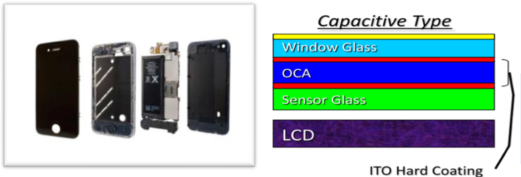
Figure 1. (L) Typical Smart Phone Construction, including Touch Screen Panel, which by itself can consist of (R) 3-5 layers of Glass/Plastic constructions.
