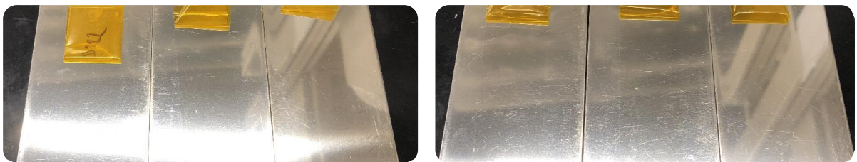
Figure 7: Heat resistance at 260^{\circ}\text{C} BTX PSA (left) & heptane PSA (right)
