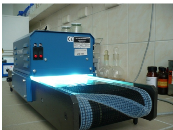
Figure 2. UV lamp with transmission belt
