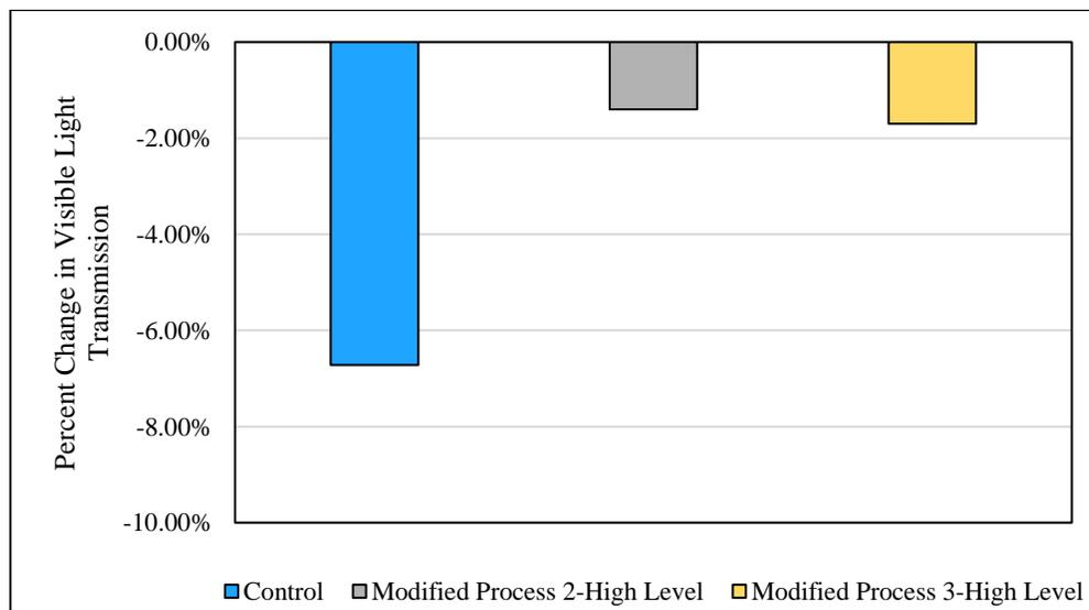
**Figure 4.** Water Whitening Resistance Testing of Modified Emulsion Polymerization Process and High Functional Monomer Loading Results
