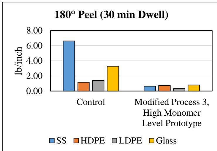
**Figure 7.** 180° Peel Values Comparison of Prototype and Control Adhesives
