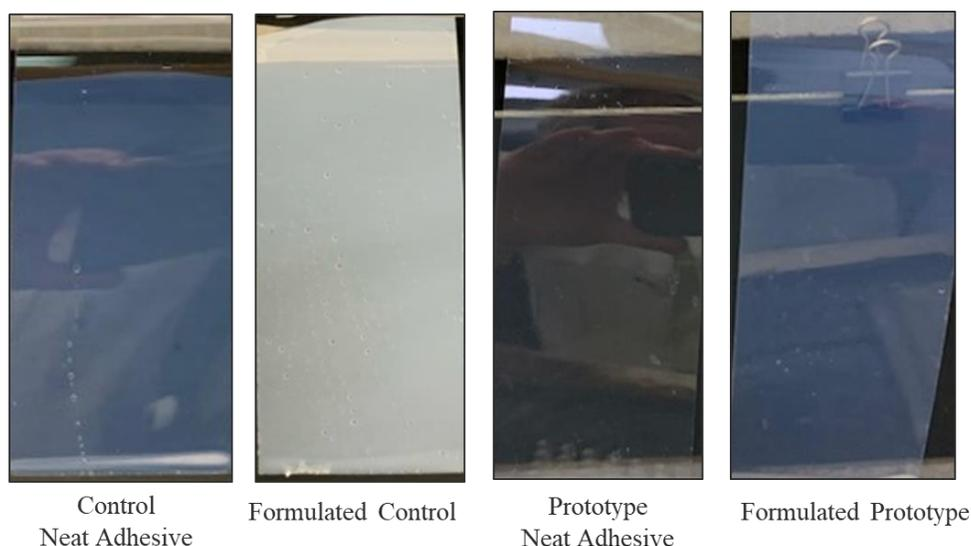
**Figure 10.** Pictures of Water Whitening Testing Results and Comparison of Neat and Formulated Adhesive Prototype
