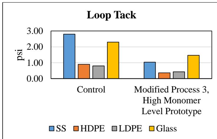
**Figure 8.** Loop Tack Values Comparison of Prototype and Control Adhesives
