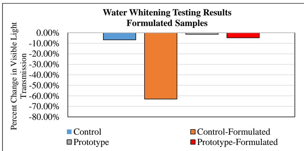
**Figure 11.** Water Whitening Testing Results and Comparison of Neat and Formulated Adhesive Prototype
