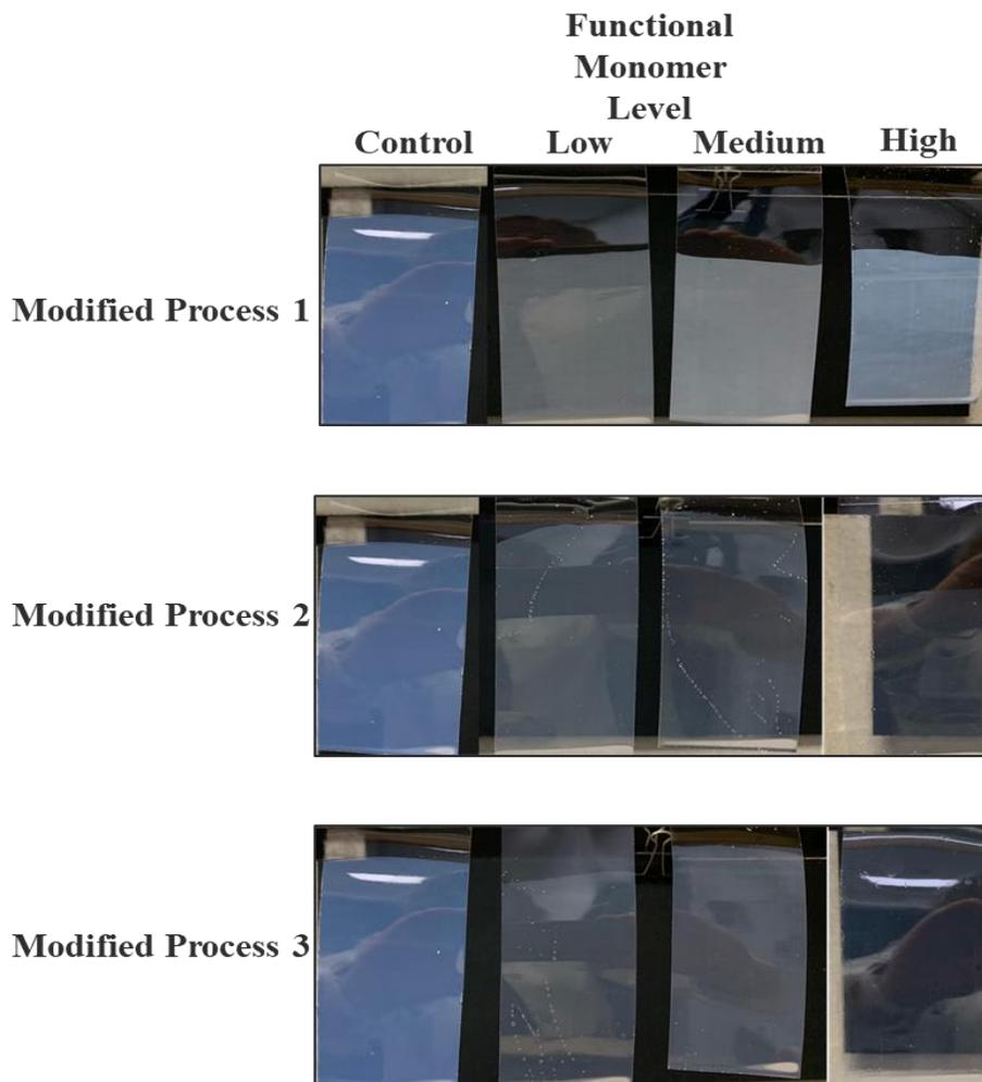
**Figure 3.** Pictures of Water Whitening Testing Results of Functional Monomer Incorporation with Modified Emulsion Polymerization Processes
