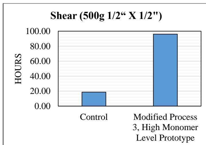
**Figure 9.** Shear Values Comparison of Prototype and Control Adhesives
