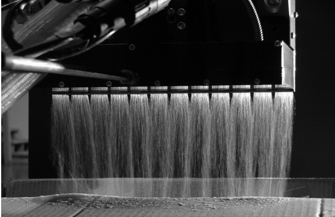
Figure 4. View of the hot melt being sprayed from a 12” wide spray head
