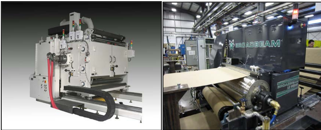
Figure 4. Industrial EB processor (150 to 300 kV) compared to new generation lower (80 to 150 kV) electron beam unit.
