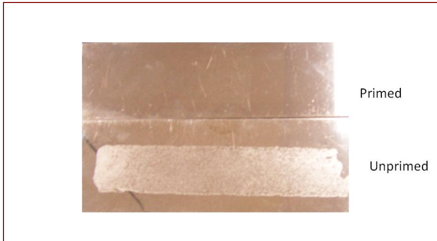
Figure 1: Residues on Stainless Steel Panels
