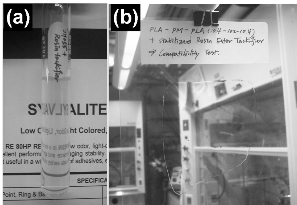
Figure 2. Compatibility tests. (a) a mixture of PLA-PM-PLA(10-100-10)/rosin ester (RE) tackifier in toluene, and (b) a transparent film from the PLA-PM-PLA(10-100-10)/RE tackifier. Reprinted with permission from Shin, J.; Martello, M. T.; Shrestha, M.; Wissinger, J. E.; Tolman, W. B.; Hillmyer, M. A. Macromolecules 2011 , 44 , 87-94. Copyright (2011) American Chemical Society.
