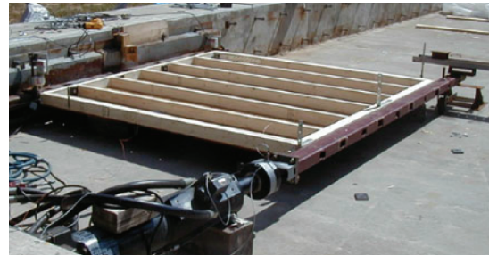
Figure 5. Photograph of the seismic racking setup, showing the hydraulic actuator used to control displacement.
