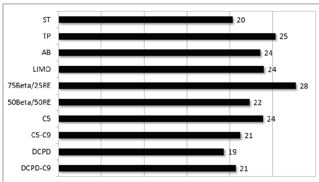
**Figure 3:** 180° Peel on SS (N/25mm) – SIS adhesive
