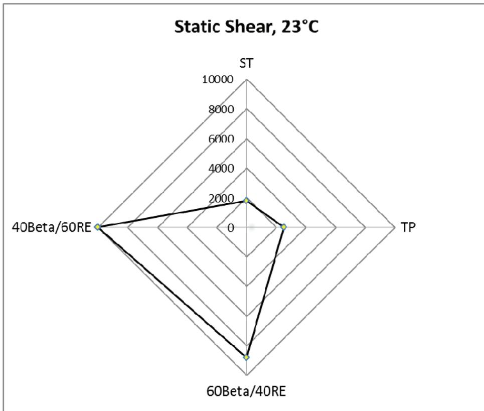
Figure 8: Static Shear - SBS adhesive
