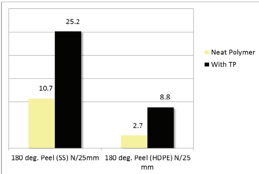
**Figure 16:** Peel on SS and HDPE with TP in Acrylic PSA
