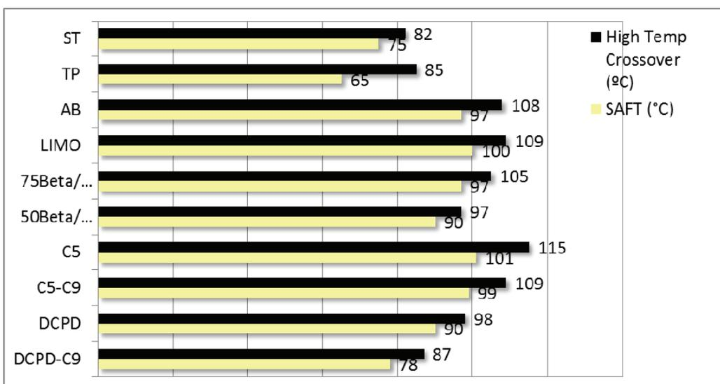
Figure 5: SAFT, G'/G'' Crossover temperature, and Static Shear\* - SIS adhesive
