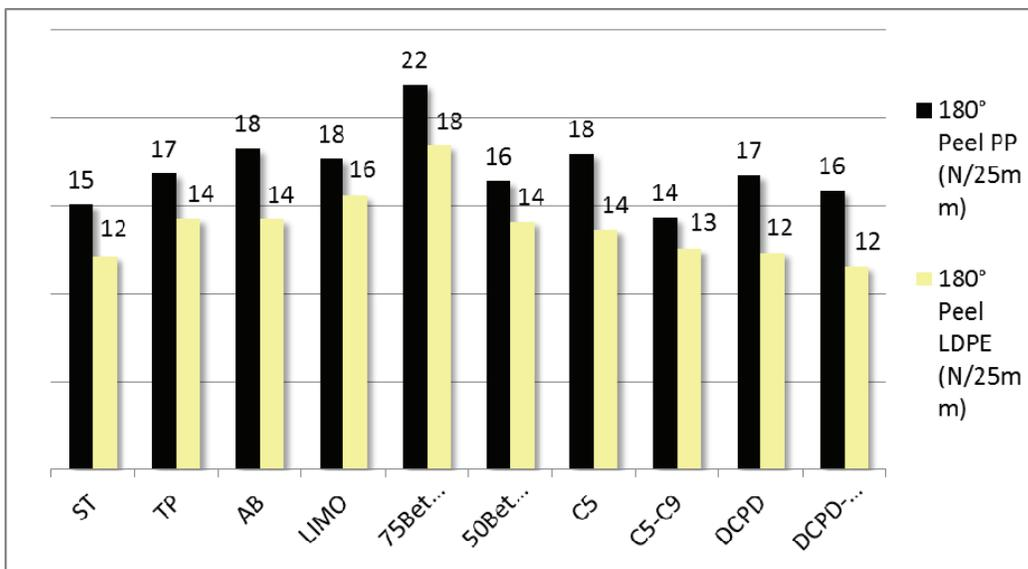
Figure 4: 180° Peel on Polypropylene and LDPE – SIS adhesive
