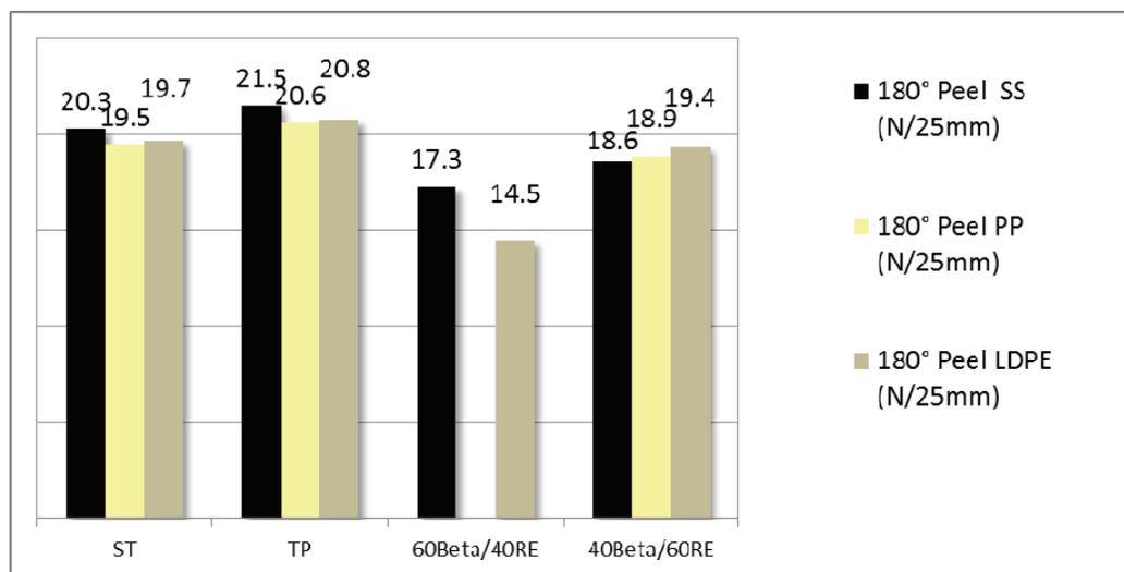
Figure 6: 180° Peel on SS, Polypropylene and LDPE – SBS adhesive
