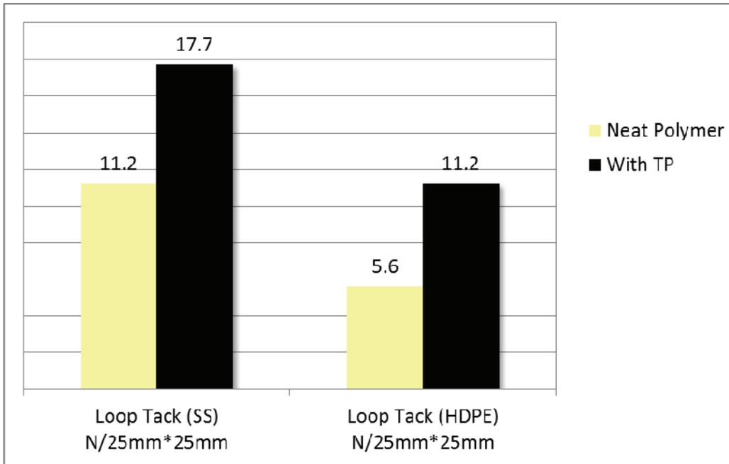
**Figure 15:** Loop Tack on SS and HDPE with TP in Acrylic PSA
