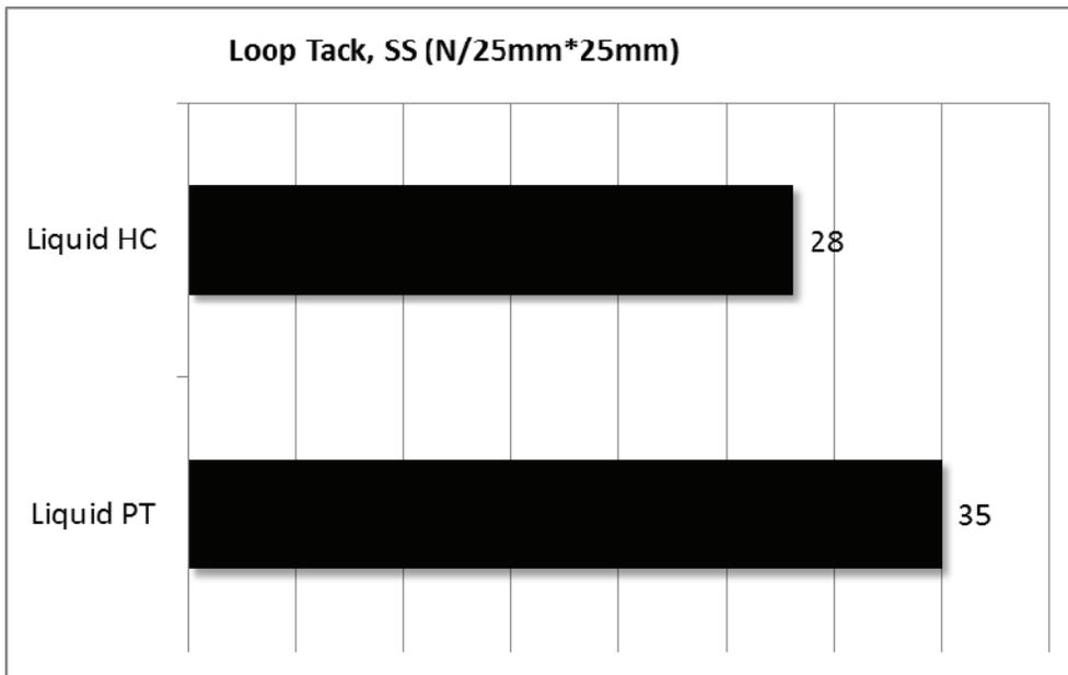
Figure 18: Loop Tack on SS with SIS label adhesive
