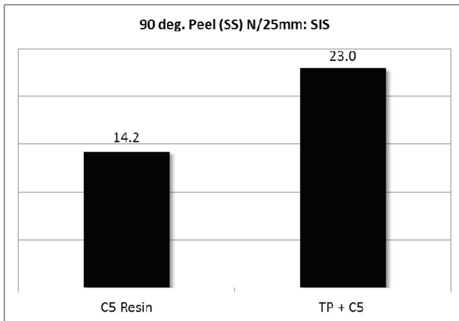
**Figure 12:** Peel on SS with TP as co-tackifier
