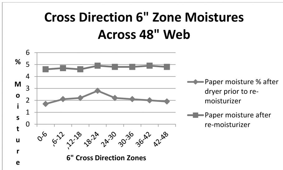
Figure IX: Web Profile Moisture Before and After Re-Moisturizer
