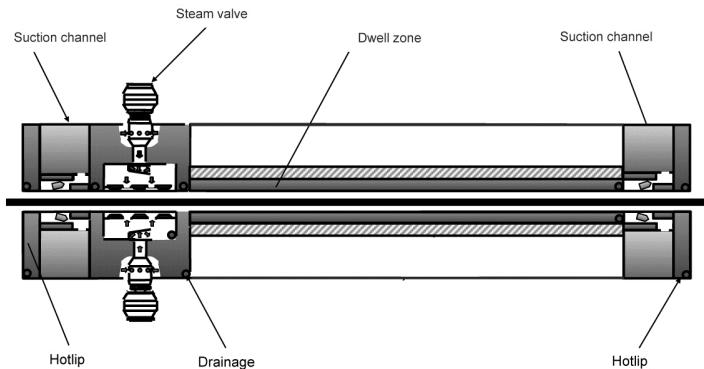
Figure II: Cross Direction Steam Re-Moisturizer
