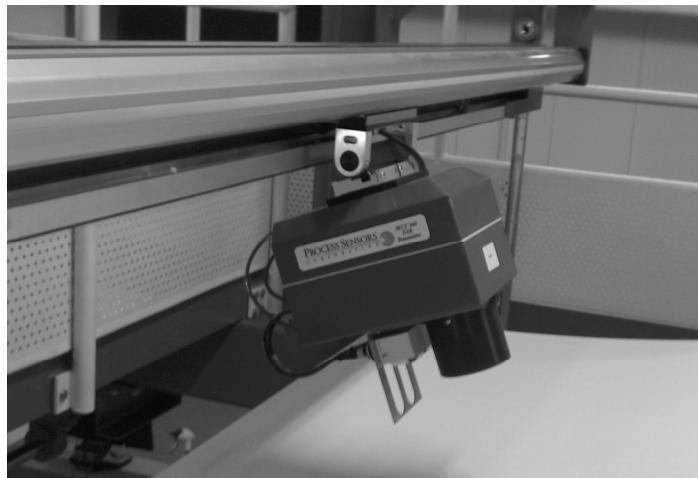
Figure VI: NIR Moisture Transmitter On Paper Web
