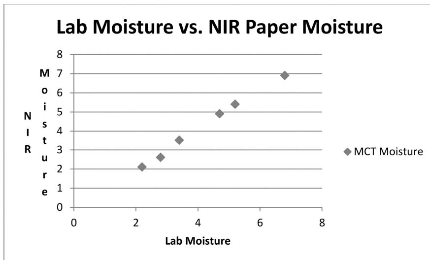
Figure X: Paper Moisture Measurement Comparison
