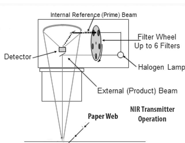
Figure V: Workings of an NIR Transmitter
