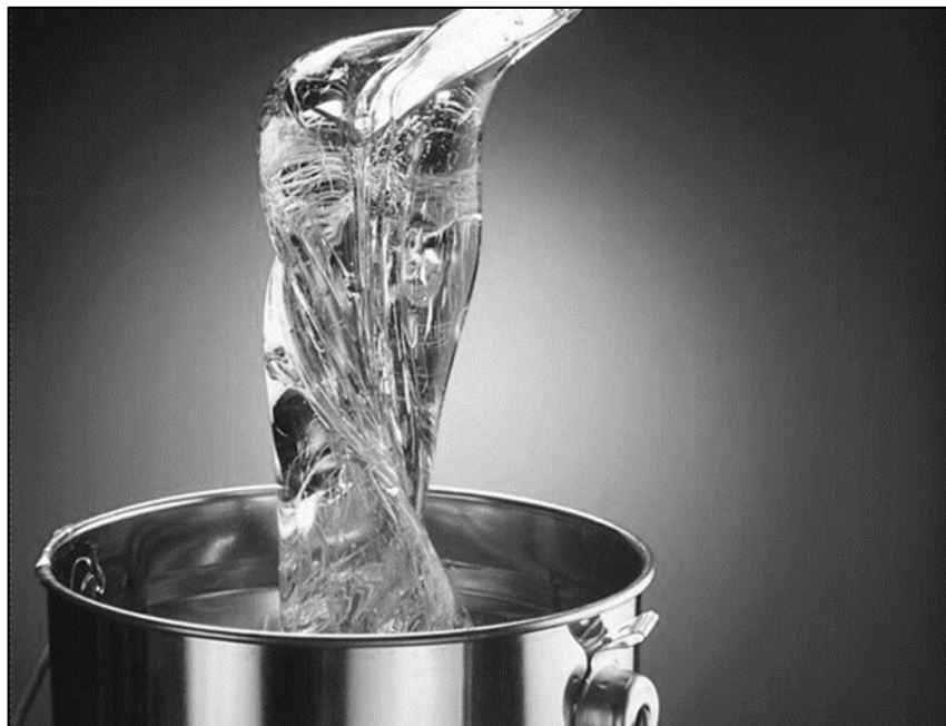
Figure 1. Sample of an acrylic UV-hotmelt in molten stage
