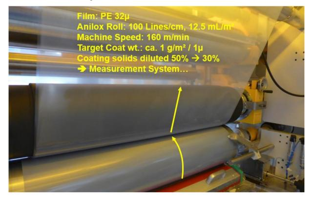
The white light interferometer coat weight measuring system returned a pleasingly flat cross direction coat weight profile despite variations in substrate thickness.
