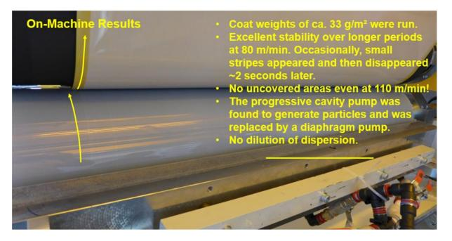
Summarising, the patience and tenacity to find a solution paid off. Elimination of high-shear hot spots was the key to success, enabling the targets for coat weight, stripes and speed to be met or even exceeded.
