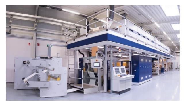
The machine used to test these conditions was a pilot coater with a working width of 1050 mm and a speed range of 2.5 - 500 m/min. At the front end, a single roll unwind system passes the web to a conditioner for normalising substrate conditions. After this, the option of web cleaning or corona treatment up to 16 kW is possible. The coating section houses a cartridge-type changeover system. Coating methods include, amongst others, roll coater, comma bar, gravure and dual layer slot die.
