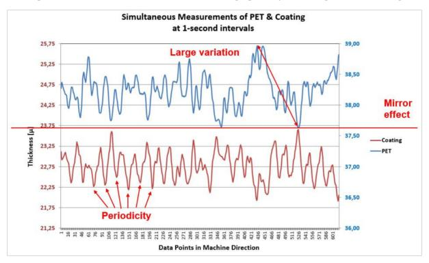
As we would expect, when we are using a calibrated gap to coat, the coating layer becomes thicker when the substrate is thinner and vice versa. The graph shows a mirror-like behaviour, confirming the theory. Interesting to note is that the swing in PET thickness does not correspond to an equivalent swing in coating thickness – the latter is larger. This, and the presence of periodicity, suggest that other factors are in play.
