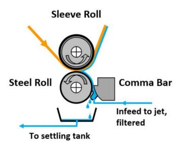
On-machine testing showed that the concept worked extremely well. Without any dilution of the adhesive, 33 g/m<sup>2</sup> dry coating was applied at 80 m/min for longer periods. No deficiencies in roll coverage were observed even at 110 m/min. Very small stripes appeared now and again, but were short-lived, disappearing after ca. 2 seconds. A diaphragm pump was used for adhesive supply, after a progressive cavity pump proved to be a source of particles.
