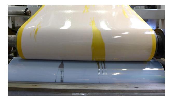
The idea arose to force-feed the roll surface with a kind of jet. This was designed and built to seal with the comma bar and have an adjustable gap to the transfer roll for optimising air exclusion and maintaining jet pressure (ca. 100 mbar).
