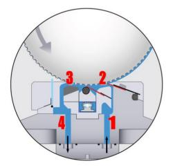
Although a pressurized gravure system ① can handle many coating tasks and has the advantage of low (or no) backflow, air exclusion becomes difficult at higher speeds and /or finer gravure required for low coat weights.
