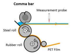
In the current example,  $23 \ \mu m$  of a viscous fluid was applied to a  $38 \ \mu m$  PET film. The white light interferometer allows us to measure both substrate and coating layer simultaneously. Exporting the data into a spreadsheet enables us to show the variations graphically and recognise trends at a glance.
