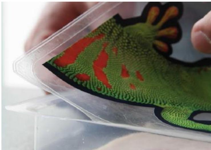
**Figure 1.** Hot melt pressure-sensitive adhesive layer as part of the co-extruded blown film
