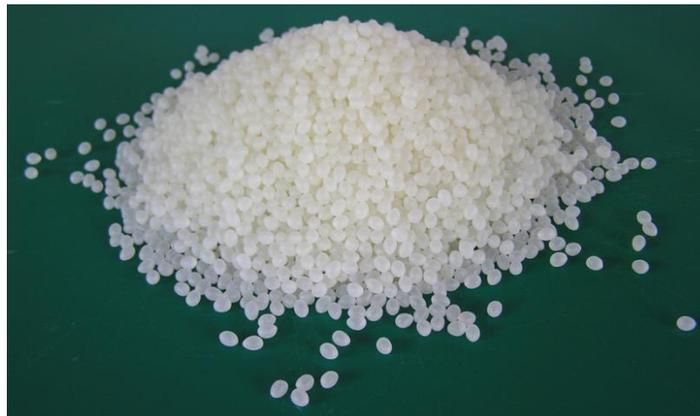
**Figure 12.** Free-flowing pellets of an extrudable hot melt pressure-sensitive adhesive product
