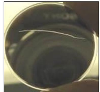
**Figure 17. Damage to the optical window on a UV radiometer such as this scratch, can result in improper measurements.**
