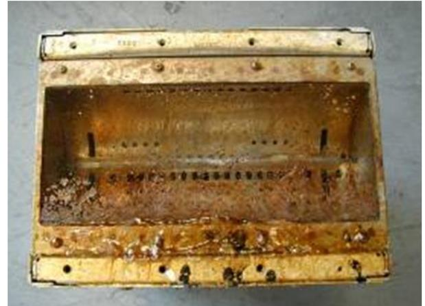
**Figure 16. Neglecting to clean reflectors causes corrosion and contamination. This reduced UV output and may affect some wavelengths more than others.**
