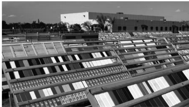
Most exposure racks are made from aluminum, and can be easily adjusted to any angle of exposure.
