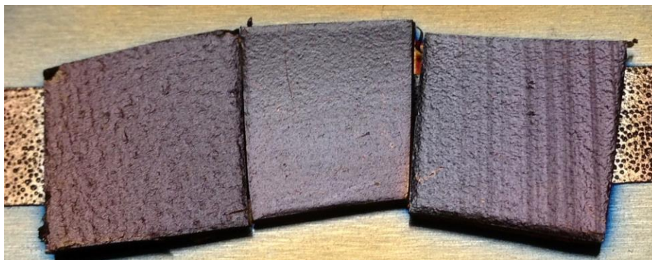
Figure 2: HDPE samples showing differences in surface texture of Au/Pd coated bottles. From left to right, jug, tan bottle and flame treated. The differences in surface texture are apparent when the coated samples are lit obliquely.
