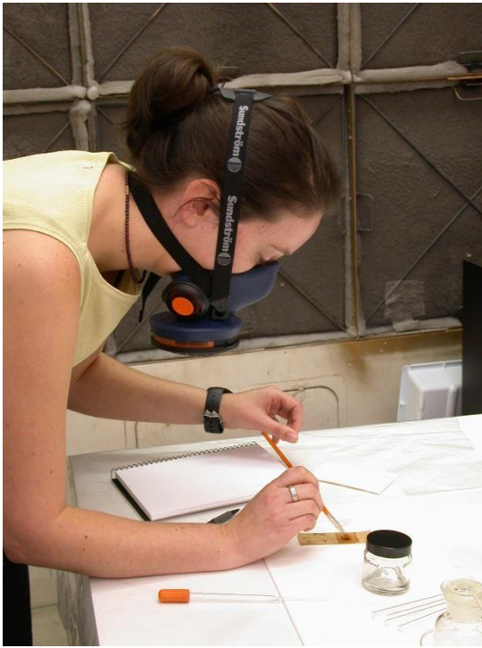
Figure 1. A conservator applies an organic solvent to a test sample
