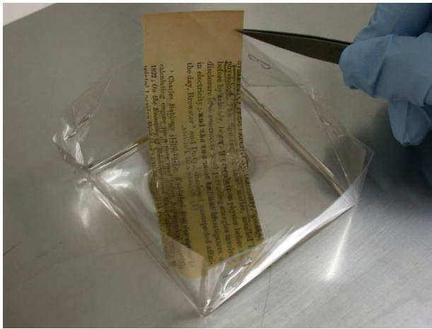
Figure 2. The sample is immersed in a solvent bath
