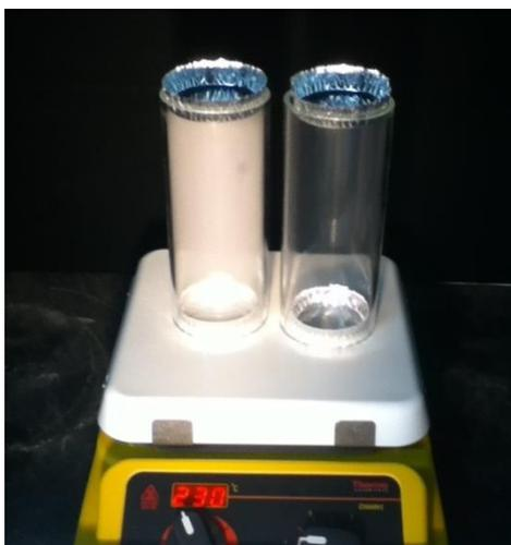
**Figure 7.** Smoke generated by heating coating baths containing conventional CRP (left) and high efficiency CRP (right). Note: Test results. Actual results may vary.
