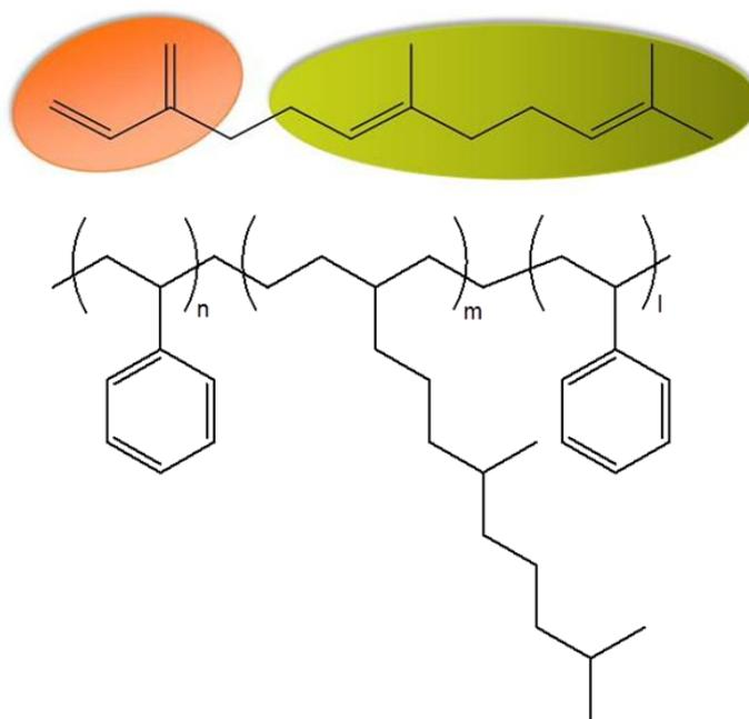
**Figure 1.** Chemical structure of  $\beta$ -farnesene and hydrogenated styrene farnesene copolymer (HSFC)
