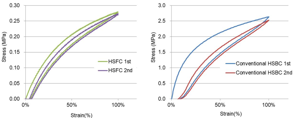
**Figure 4.** Two cycles of stress-strain curve of HSFC and conventional HSBC (SEPS) showing their hysteresis losses
