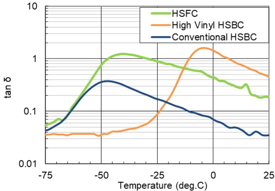
**Figure 3.** Temperature dependence of loss tangent of HSFC compared to HSBCs
