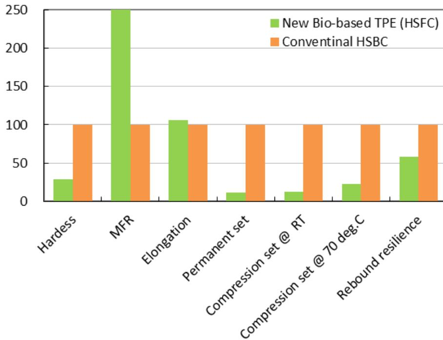
**Figure 2.** Comparison of HSBC and HSFC in basic properties
