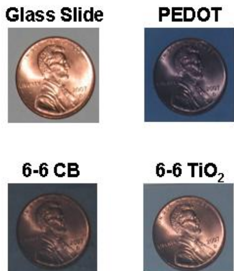
Figure 9. Images of 12-bilayer PEDOT-based assemblies on glass slides placed over a penny to highlight the disparity between films containing carbon black or TiO 2 nanoparticles in their final 6 bilayers (adapted from Ref. 12).
