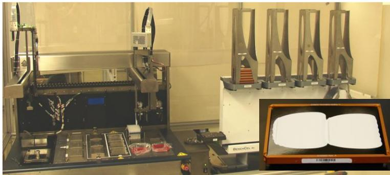
**Figure 6:** Symyx Coating Station with ability to coat 1-8 coatings on a single test panel. Coatings can be made at different thicknesses and on different test panel materials.
