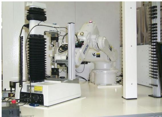
**Figure 7:** (a) Symyx Tack Station with automated probe tack test. Probe tack is performed using  $\frac{3}{4}$ " diameter spherical probes which can be different materials such as steel, glass etc. (b) Automated Peel tester with ability to perform 180 degree and 90 degree peel test on different types of test panels (HDPE, Glass, Stainless Steel etc.)
