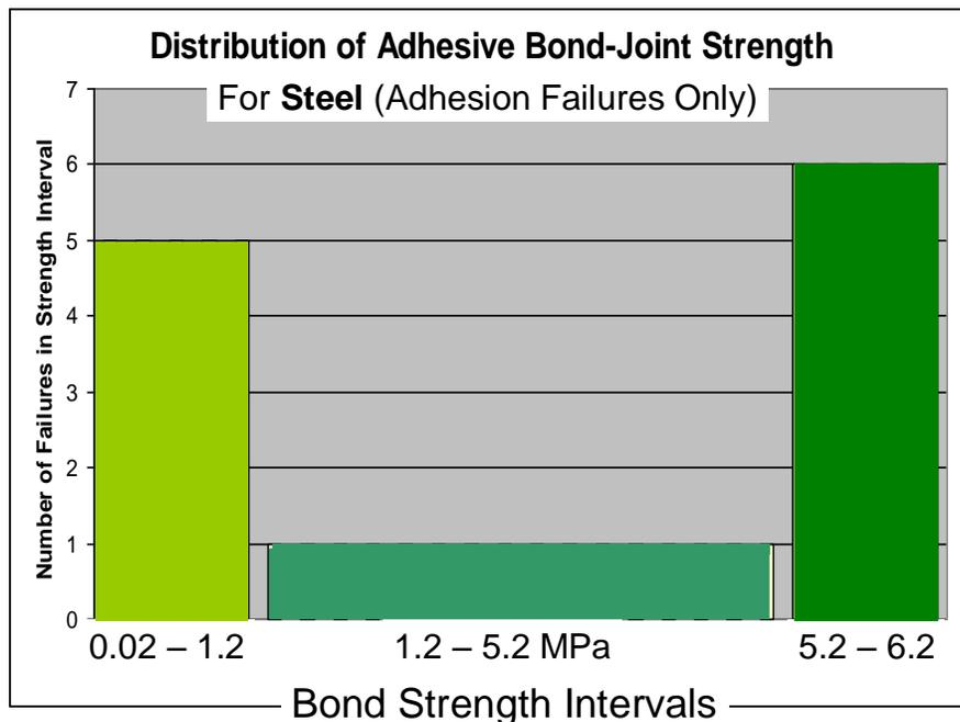
Figure 7(c). Adhesive bond-joint strength distribution is bi-modal for all failure modes in steel bond joints that survive preparation.
