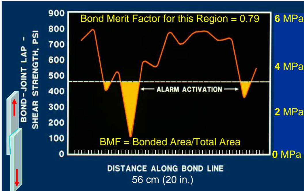
Figure 4. Bond-strength profile along a typical adhesively bonded lap joint.
