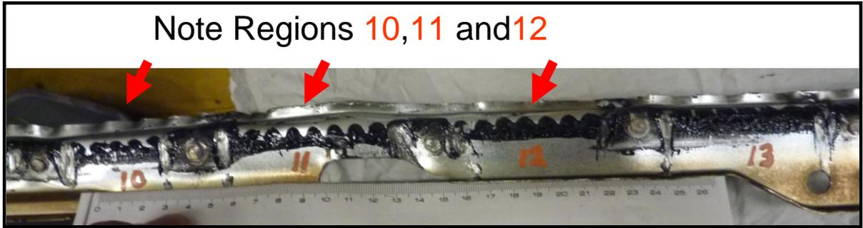
Figure 8. Disassembled weld-bond joint from sheet-steel vehicle body showing unintended wavy adhesive pattern in regions 10, 11 and 2, with spot weld nuggets separating regions.
