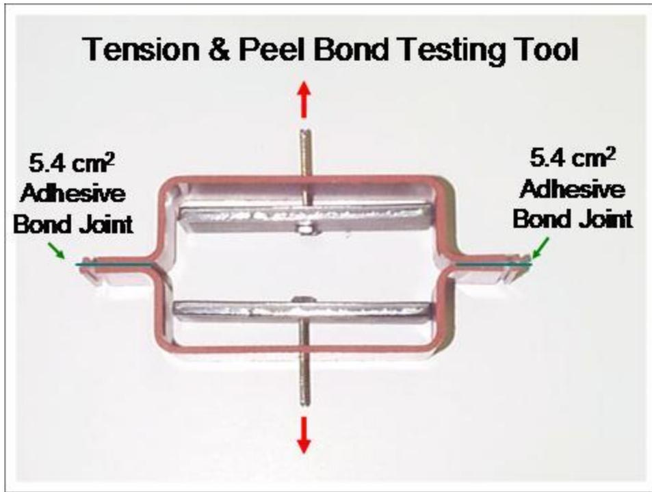
Figure 5. Tool and specimen for testing bonds in box sections by tension-peel loading.
