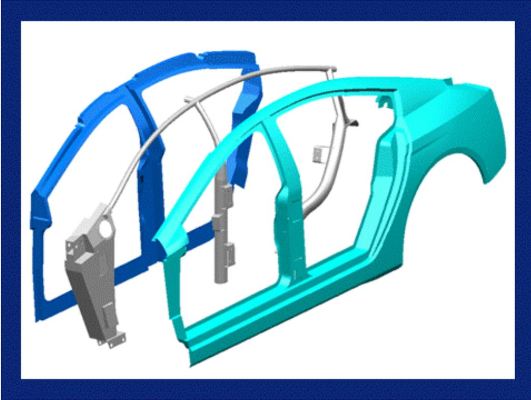
*Figure 3. An example of joining requirements placed on adhesives to assure the high-quality performance and appearance of such a multi-material vehicle body component made from polymer composite, metal and thermoplastic materials.*
