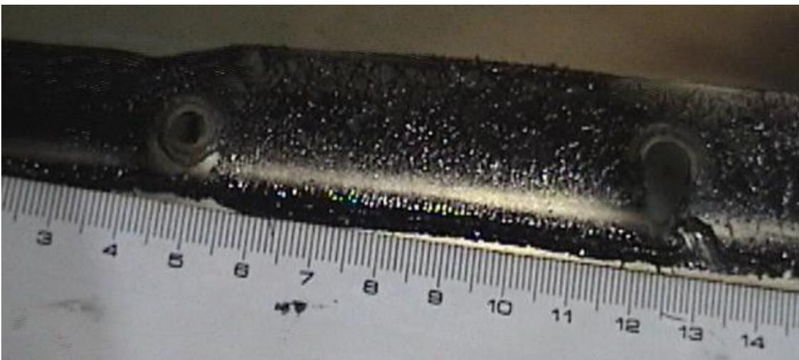
Figure 10. This narrow region of thinned adhesive along the bond joint does not adversely impact bond joint performance after curing.
