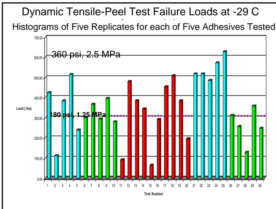
Figure 6. Adhesive bond failure-load data from tension-peel testing six different adhesives, using five replicates for each adhesive, at low temperature.
