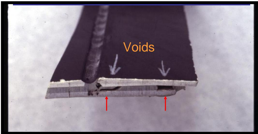
*Figure 11. Adhesively bonded fiber-reinforced plastic lap joint showing voids caused by missing adhesive.*
