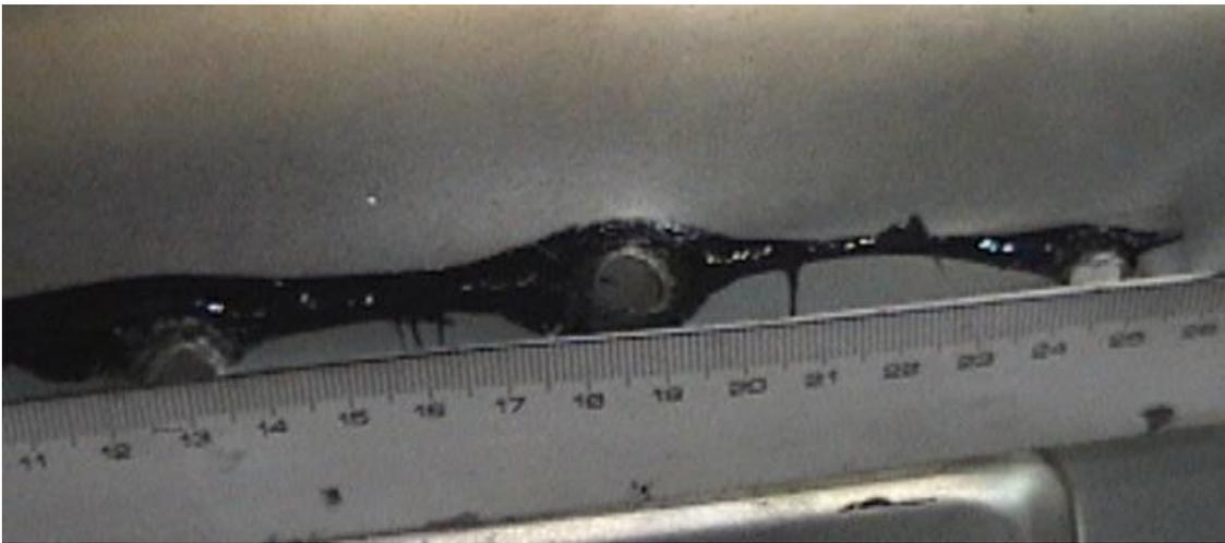
Figure 9. Narrowing adhesive in regions between spot welds
