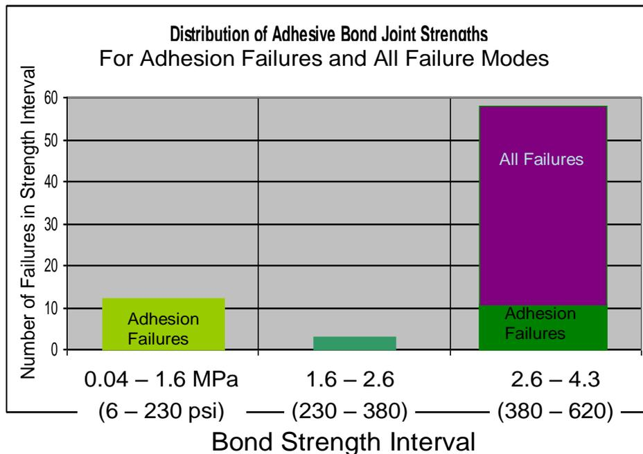
Figure 7(b). Adhesive bond-joint strength distribution is bi-modal for all failure modes in fiber-reinforced plastic bond joints that survive preparation.
